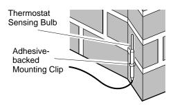
Figure 49 - Locating Thermostat Sensing Bulb on Masonry Fireplace
